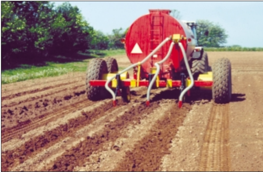
Liquid manure injection system.
